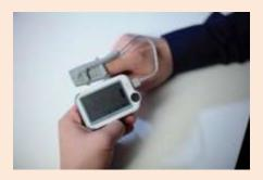
A group of engineers at the Indian Institute of Technology (IIT), Madras, has developed the algorithm for a medical-grade, wearable device called VinCense. The device can be used for unobtrusive monitoring of vital signs including pulse-rate, oxygen saturation, respiratory rate, skin temperature and blood pressure.
